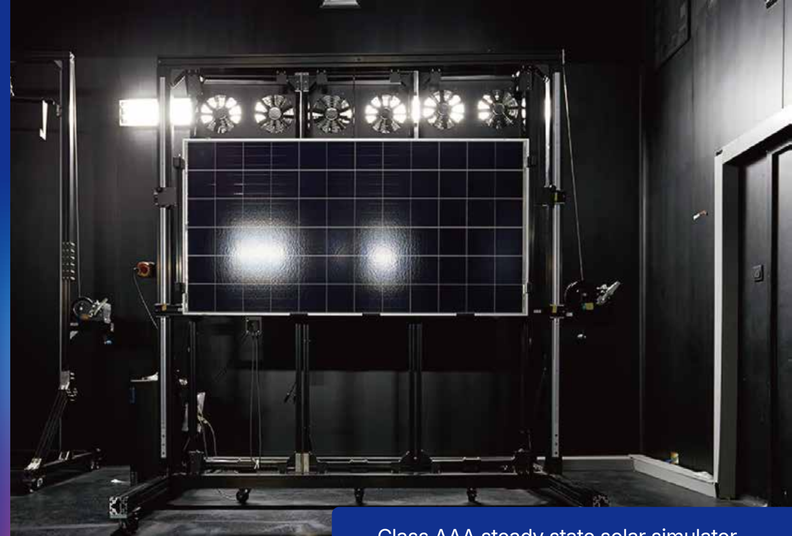
Class AAA steady state solar simulator
